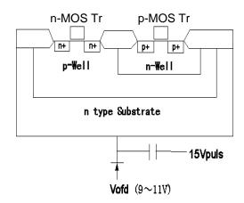
Figure 8. Cross section of CMOS
