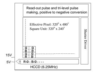
Figure 7. Block Diagram of Dual Pixel CCD
