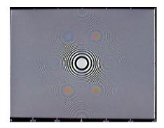
Figure 3. QVGA Image of CZP chart by Conventional Sensor
