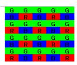
Figure 2. An example of color filter arrangement for dual pixel sensor
